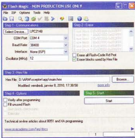
Figure 4. Configuring Flash Magic. The communications parameters are the most important ones. For programming, the serial port speed must not be above 38,400 baud. For the terminal, you can choose a higher speed.
