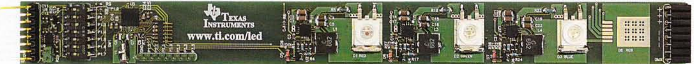
Figure 7. DMX receiver PCB.
