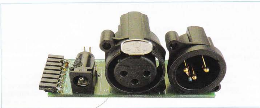
Figure 6. Adapter board fitted with XLR connectors and a power connector.
